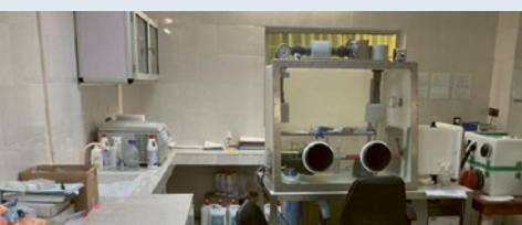
New Glovebox for secure inactivation at LFHB, Cotonou, Benin (Photo ©Nathalie Vielle, BNITM)
