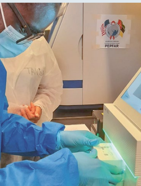
Starting the iSeq100 sequencer with SARS-CoV-2 samples for whole viral genome sequencing. (Photo ©Nalia Ismael)
