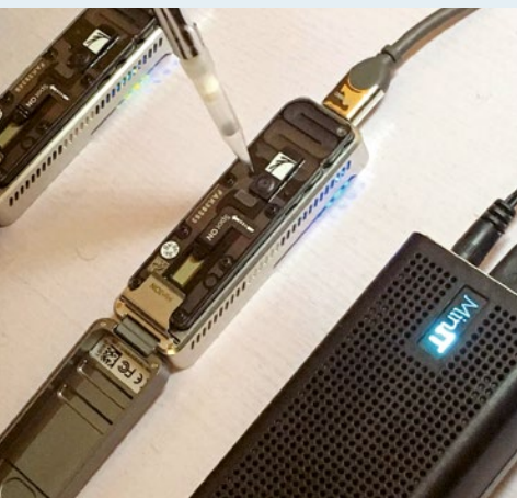
Adding the sequencing library into the Nanopore sequencer (MinION, Oxford Nanopore) which has a size of a chocolate bar
